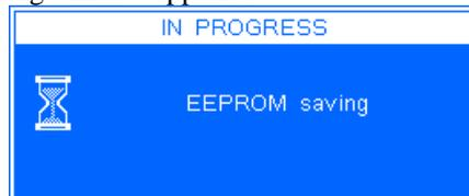
This operation takes a few seconds. Then the following message will be displayed to indicate that you must toggle the calibration jumper to its initial position (normal mode position):
