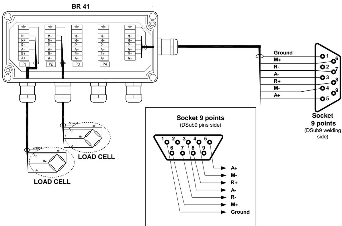
3°/ Before connecting the load cell cable on the M1 socket of the IDL, you must verify the following impedances on the DSUB 9 points connector:
